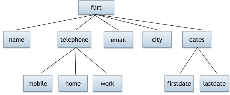
Because of the distinct, tree-like structure and similarity to object-oriented systems, computers are able to unambiguously recognise the data structure when reading an XML document.
